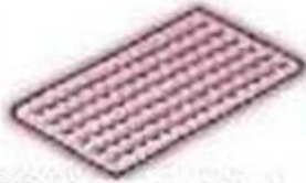
CSP (Underside View)
