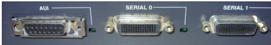
Figure 3-2: Most WAN interface or network interface connections are managed through AUI and serial ports.
