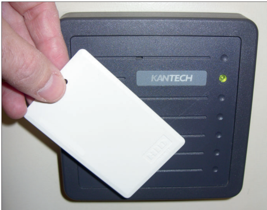
Figure 4-3: A standard proximity card and card reader.
