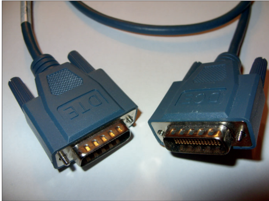
Figure 5-3: A router-to-router back-to-back serial cable.
