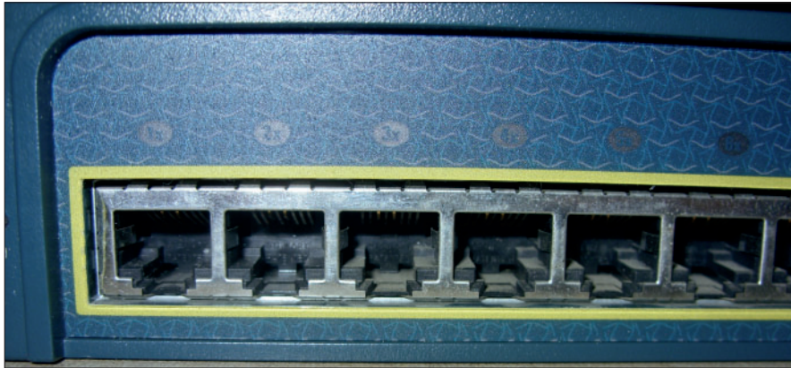
Figure 2-3: The most common port on a switch is the RJ45 port.
