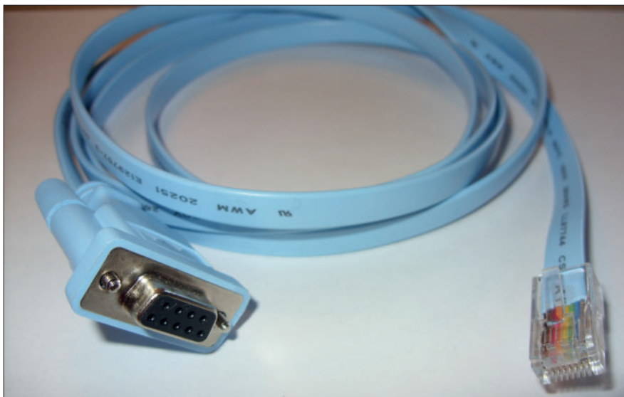
Figure 5-2: A Cisco rollover cable.
