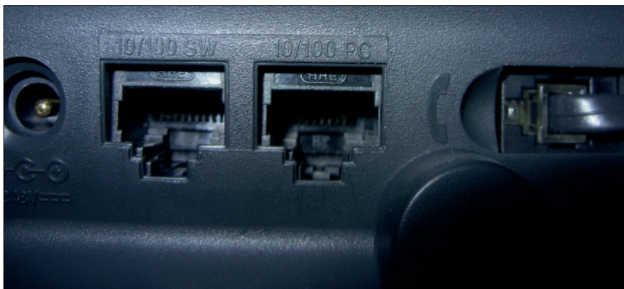
Figure 5-3: The two-port switch integrated into Cisco IP phones.
