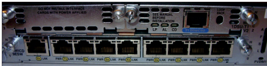
Figure 3-3: A T1 WIC card and 8-port switch installed in HWIC interface ports.
