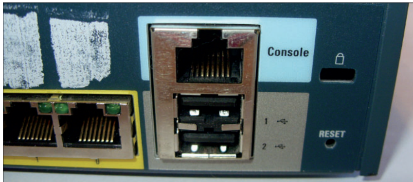
Figure 5-4: Console/ serial port on your Cisco device.
