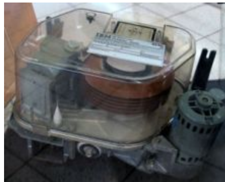
IBM 62PC "Piccolo" HDD, circa 1979 - an early 8" disk
